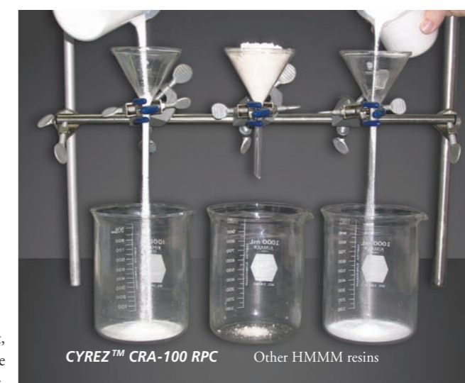
In flowability and low dust generation test, CYREZ™ CRA-100 RPC excels in performance compared to other HMMM resins.
