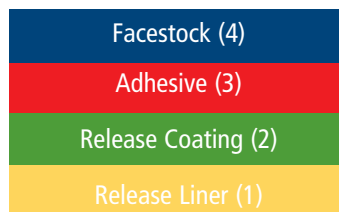
Figure 1 – Pressure Sensitive Laminate Construction (Four Elements)
